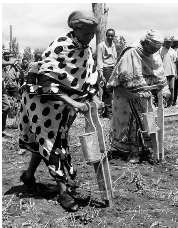
Farming in Tanzania: The hand jab planter matraca speeds up the planting process and allows farmers to work in a standing position
